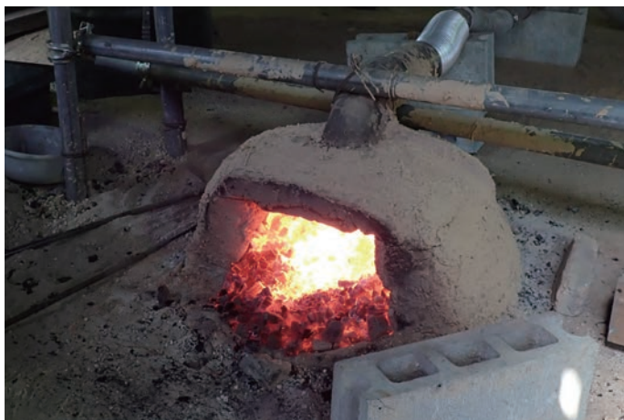
古代中国炒鋼炉の復元と実験 Restoration and Experimentation of Furnace for Iron Refining in Ancient China
